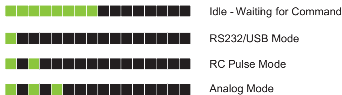
FIGURE 16. Status LED Normal Operation Flashing Patterns
